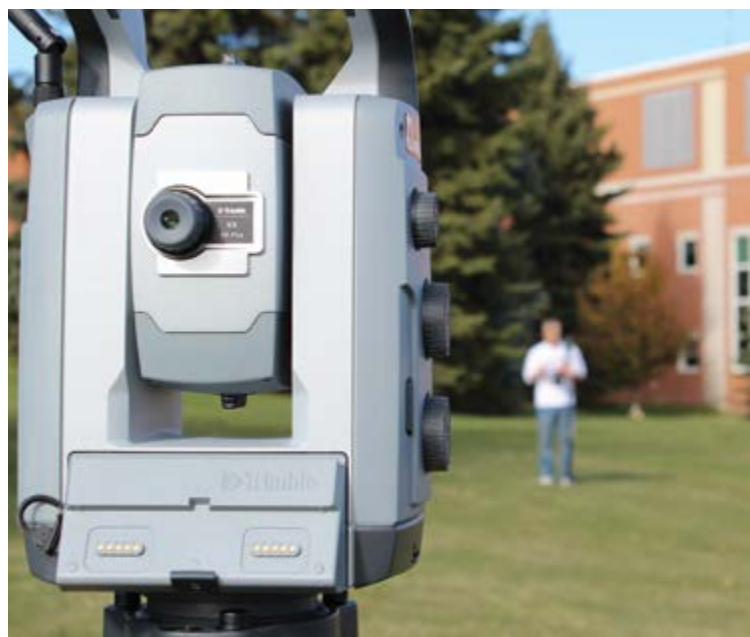
Below: Robotic Total Station provides hands-on industry experience for BSC engineering tech students.
